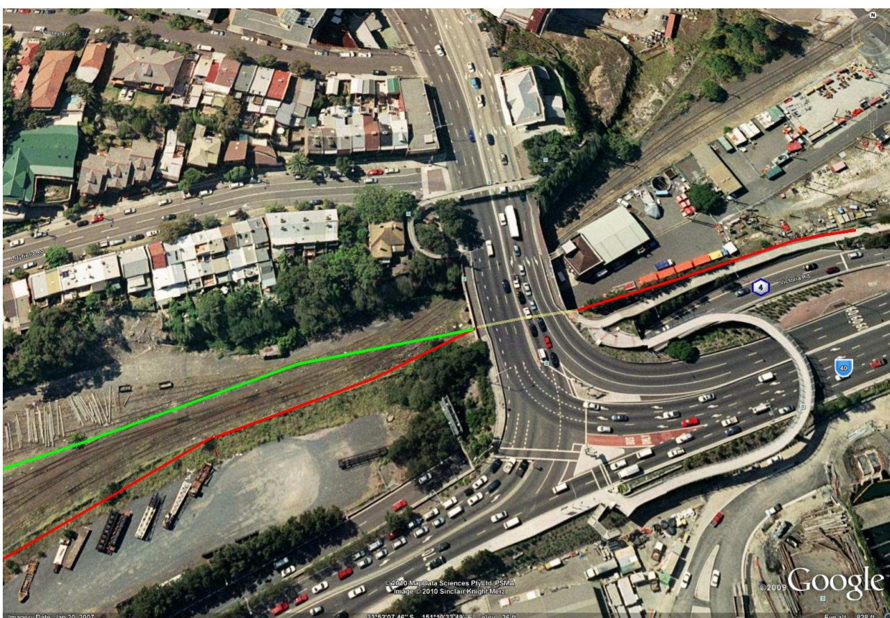
Illustration 11: Cycleway passing under Victoria Road and connecting to the Anzac Bridge cycleway
