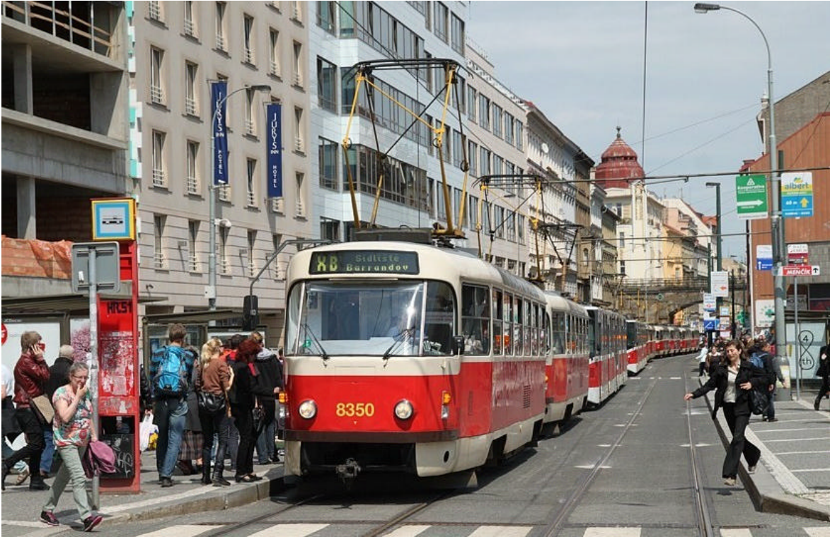
Figure 1: Trams in Prague substituting for a closed metro line during floods in 2012. This is not a tram jam, the trams are moving like a conveyor belt, something only possible with a looped line or a line split into several branch lines at both ends with each branch line in turn having reversing stubs of sufficient capacity. In events like this, traffic light priority is also given to the trams.
