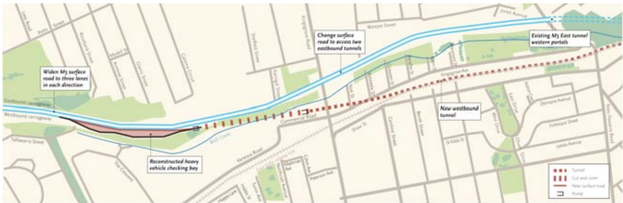
Figure 8.2 Slot tunnel alignment
